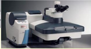
Figure1: FTIR and Raman spectrometer Thermo Scientific
